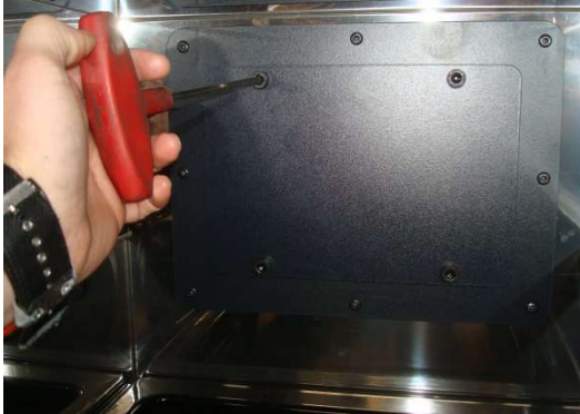
Figure No.21 - Access to the screws to remove the hatch cover
