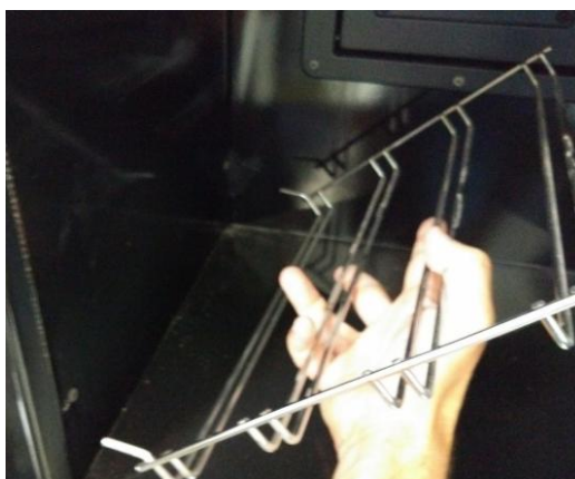
Figure No.22 - Removal of the brackets and self-cleaning sides
