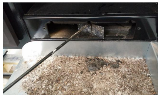
Figure No.21 - Accesses via which to clean the flue socket.
