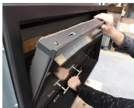
Figure No.41 - Hold the door firmly with both hands as you lower it
