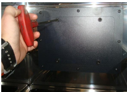
Figure No.17 - Access to the screws to remove the hatch cover
