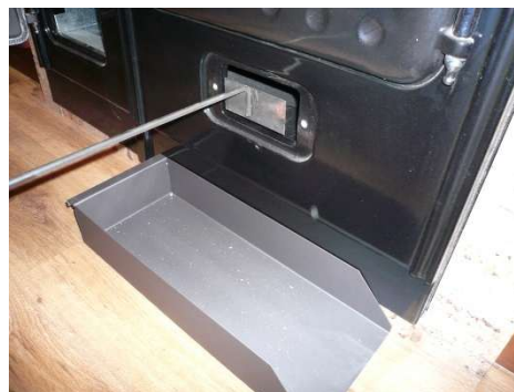
Figure No.18 - Accesses via which to clean the flue socket.
